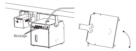
When the joint of the terminal liquid tank is not connected to the pipeline, it is necessary to put a blockage, otherwise the liquid will easily overflow.
